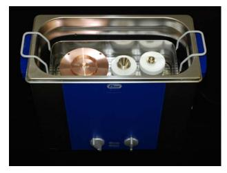
The cone's tip is inverted into fixture. The container can be filled with Citranox, nitric acid or a cleaning solution of your choice. Using this method, HNO<sub>3</sub> concentrations as high as 10% can be used to clean platinum cone tips without damaging the nickel or copper base. When cleaning nickel cones limit your nitric concentration to 2%.
