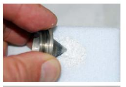
After creating a light paste with fine alumina powder, polish your cone tip using a felt pad or cotton cloth. Though the felt pad is gentle, do not apply excessive pressure directly on the tip of the cone. Certain skimmer cones are particularly prone to blunt force trauma due to their thin walls and sharp edges.
