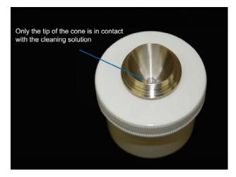
Using this simple cone fixture it is possible to efficiently clean the cone's analytical zone without degrading the rest of the cone unnessesarily. This is particularly useful for Pt tipped cones and cones with exposed copper bases.
