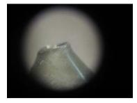
**Delicate skimmer cone damaged in an attempt to clear orifice with metal wire:** This cone is now functionally unusable. Many skimmer cones have very thin walls with sharp edges. Any attempt to force a probe (metal, wood or plastic) through this delicate orifice may alter the cone dimensions outside manufacturer specifications
