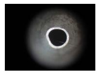
**Platinum cone damaged from mishandling**: Since the metal is in good condition; neither annealed nor chemically degraded, it can be easily refurbished. Our free Pt refurbishing process will reform the cone to within the manufacturer's original specifications.
