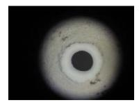
Skimmer cone with a simple salt build up: Sonicating in  $dH_2O$  or dilute  $HNO_3$  (<1%), after soaking in Citranox can usually clean these cones effectively. Dry according to instructions.
