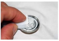
After creating a light paste with fine alumina powder, polish your cone tip using a felt pad or synthetic, lint free cloth. Though the felt pad is gentle, do not apply excessive pressure directly on the tip of the cone. You want to remove build up without changing the geometry of the cone tip.
