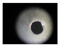
**Platinum cone chemically degraded beyond repair:** Here the cone has been made brittle and porous. This cone is ready for Pt reclamation. For the current *Pt Reclaim Credit* values go to the **Library and Resources** section of our web site.
