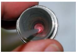
For optimal cleaning of the cone orifice Spectron recommends using diamond paste and a foam tipped cleaning stick. These sticks simplify the effective cleaning of the most important region of the analytical zone.
