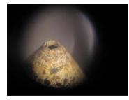
**Typical skimmer cone with oxide buildup:** We recommend soaking this cone in Citranox<sup>TM</sup> for a few hours, then sonicating for 15 min. If this does not remove all residue follow *Aggressive Cleaning* protocol. If Citranox and sonication sufficiently clean the cone, rinse thoroughly in tap water then dH<sub>2</sub>O. Dry according to instructions.
