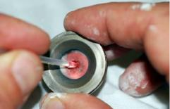
For optimal cleaning of the cone orifice Spectron recommends using diamond paste and a foam tipped cleaning stick. These sticks simplify the effective cleaning of the most important region of the analytical zone.
