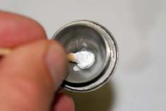
A cotton swab is very effective at cleaning the inside (concave side) of the cone. Using the same alumina paste, clean as close to the orifice as possible. By creating a point at the tip of the cotton swab it will be possible to clean residue from the inside edge of the orifice.
