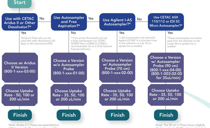
Note: Aridus II C-Flows are assembled at 110 degrees C. They can not be used for normal room temperature applications (i.e. non-desolvator)
