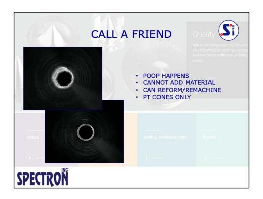
PLATINUM REFURBISHING CAN ALSO CORRECT DAMAGE CAUSE BY SLIPPERY FINGERS. IF THERE IS SUFFICIENT MATERIAL, CONES CAN OFTEN BE REFORMED AND RETURNED TO THE ORIGINAL GEOMETRIC TOLERANCES.
