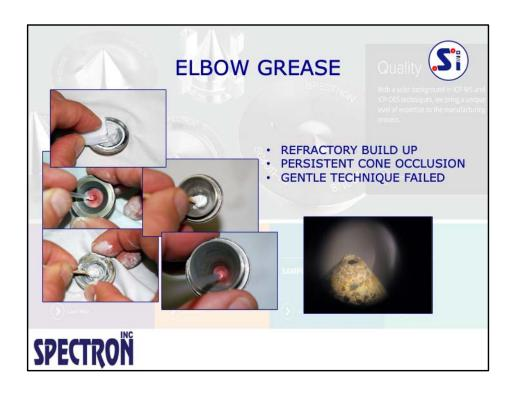
HIGH PURITY FINE ALUMINA POWDER, OR DIAMOND PASTE IS RECOMMENDED, BUT MANY HAVE USED BON-AMI™, OR SIMILAR CLEANING ABRASIVES. CREATE A PASTE ADDING DH2O TO ABRASIVE POWDER AND FIRST CLEAN THE INSIDE ANGLE OF THE CONE BY APPLYING PASTE WITH A COTTON SWAB. THE TOP ANGLE (TIP) OF THE CONE, ESPECIALLY THE SKIMMER CONE REQUIRES A MORE DELICATE APPROACH. WITH COTTON SWAB, OR GAUZE APPLY PASTE TO TOP ANGLE BUT NEVER APPLY PRESURE DIRECTLY ON TIP.
