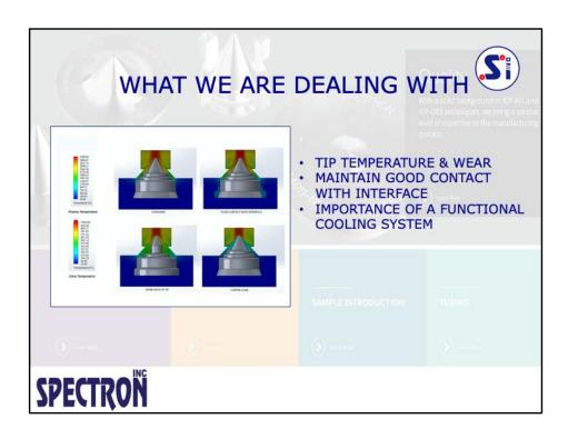
THE MODEL DISPLAYED REPRESENTS VARIOUS PARAMETERS THAT AFFECT TIP TEMPERATURE AND THEREFORE PERFORMANCE AND WEAR. GOOD OR POOR CONTACT WITH THE INTERFACE, POOR INTERFACE COOLING, ALTERNATE MATERIALS AND CONE MASS ALL PLA Y A ROLE IN CONE TIP TEMPERATURE.
