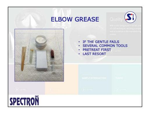
IF CHEMICAL CLEANING IS UNSUCCESSFUL AT REMOVING MATERIAL OCCLUDING THE ORIFICE OF THE SAMPLE, OR SKIMMER CONE THERE ARE WAYS TO GENTLY CLEAN MECHANICALLY.
