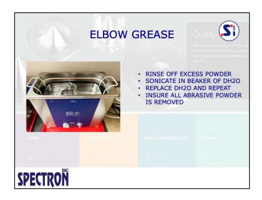
FOLLOWING A THOROUGH RINSING WITH SQUIRT BOTTLE, OR EQUIVALENT, PLACE CONES IN BEAKER OF DH20 AND SONICATE FOR 5-10', THEN REPEAT WITH FRESH DH2O. DRY WITH N2, OR AR
