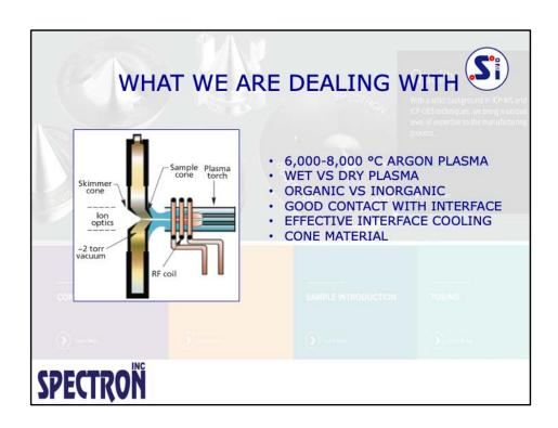
AS WE KNOW THE ICP IS AN AGGRESSIVE ENVIRONMENT. CONE WEAR OCCURS THROUGH THERMAL AND CHEMICAL ABLATION AND THE RESULT OF VARIOUS CONE CLEANING TECHNIQUES. THIS CAN BE EXACERBATED BY SAMPLE MATRIX, OR POOR INSTALLATION AND CONTACT WITH THE WATER COOLED INTERFACE. ORGANIC MATRICES ARE PARTIUCULARLY HARD ON INTERFACE CONES
