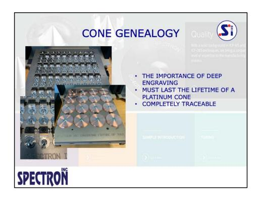
IN ORDER FOR OUR CONES TO BE COMPLETELY TRACEABLE IT BECAME NECESSARY TO ENGRAVE SERIAL NUMBERS DEEP ENOUGH TO WITHSTAND YEARS OF CHEMICAL AND THERMAL ATTACK.
