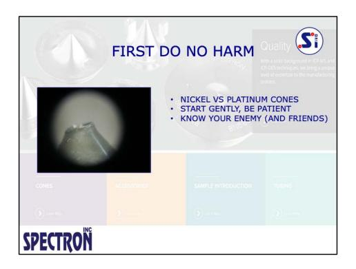
AS WITH LIGHT SOCKETS, NEVER STICK FOREIGN OBJECTS, ESPECIALLY METALIC ONES INTO THE CONE ORIFICE. THE ORIGINAL DIMENSIONAL TOLERANCES CANNOT BE HELD BY MANUAL MANIPULATION.
