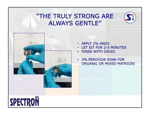
FOR INORGANIC RESIDUE, START WITH A GENTLE APPLICATION OF 2% HNO3, WITH A COTTON SWAB, AT THE BACK AND FRONT OF THE CONE ORIFICE. LET SIT FOR 2-5', WIPE OFF RESIDUE WITH COTTON SWAB, THEN RINSE WITH DH2O. FOR ORGANIC OR MIXED RESIDUE START WITH 3% PEROXIDE SOAK FOR 15'-30", THEN REMOVE RESIDUE WITH COTTON SWAB, OR CLOTH AND RINSE WITH DH2O. NEVER WIPE DIRECTLY ACROSS THE SKIMMER TIP. HOWEVER IF YOU CAN GET AWAY WITH A DH2O CLEANING PROCESS, DO IT.
