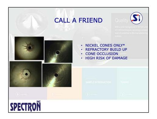
THERE MAY BE TIMES WHEN COMPLETE REMOVAL OF OCCLUSIONS ENDANGER THE INTEGRITY OF CONE GEOMETRIES. FOR PLATINUM CONES THERE IS AN ALTERNATIVE, CONE REFURBISHING. USING SIMILAR TECHNIQUES TO THE MANUFACTURING PROCESS IT IS POSSIBLE TO BRING CONES BACK TO ORIGINAL, OR NEAR ORIGINAL CONDITION. HOWEVER IT IS ONLY COST EFFECTIVE FOR PT CONES.
