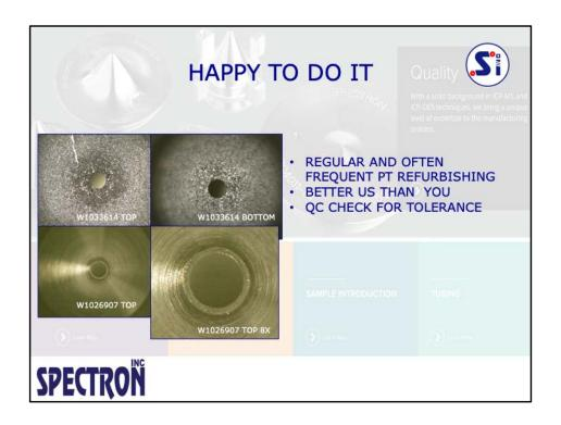
IT IS NOT UNCOMMON FOR OUR CUSTOMERS TO SEND BACK THEIR PT CONES FOR FREQUENT REFURBISHING, RATHER THAN RISK CLEANING THEM THEMSELVES, OR TO REPAIR FOR MINOR ISSUES. BOTH UPON RECEIPT AND FOLLOW REFURBISHING SPECTRON INSPECTS ALL CONES AND CHECKS THEIR DIMESIONAL TOLERANCES.
