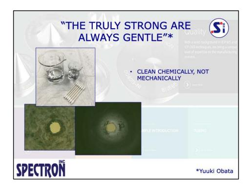
THOUGH SOME MAY SUGGEST CLEANING EXCLUSIVELY WITH DH2O, IT IS MY EXPERIENCE THAT THIS WILL ONLY WORK FOR MILD SALT BUILDUP. FOR SEVERE BUILD UP OF SALT DEPOSITS AND ESPECIALLY REFRACTORY OXIDES, OR OGANICS A SLIGHTLY MORE AGGRESSIVE APPROACH MAY BE NECESSARY.
