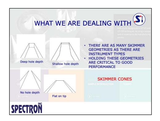
THE SKIMMER CONE IS BOTH MORE DELICATE AND MORE UNIQUE, BASED ON THE OVERALL DESIGN OF EACH ICP-MS THAN THE SAMPLE CONE. THEY ALSO PLAY A GREATER ROLE IN THE GENERAL PERFORMANCE AND QUALITY OF YOUR DATA. MAINTAINING THE ORIGINAL DIMENSIONS OF THESE CONES INSURES CONTINUED PERFORMANCE.
