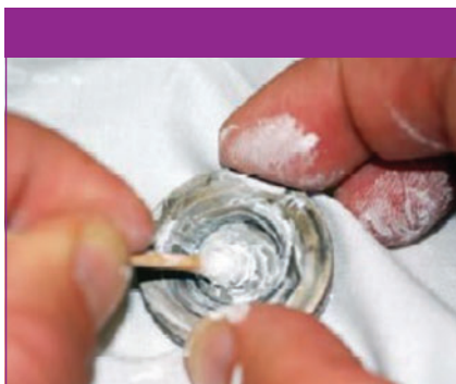
Figure 9: Showing the use of the tip of a cotton swab to clean residue from the inside edge of a cone orifice.
