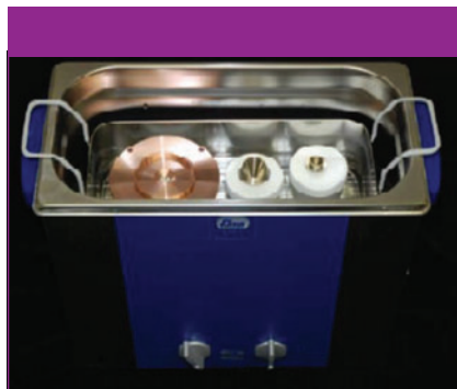
Figure 7: Cones can be cleaned in the fixture with a cleaning solution of choice and sonicated if desired.
