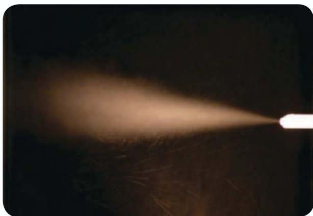
Aerosol of 25% w/v NaCl solution. (left), and nebulizer tip (right) – both after 4hrs.
