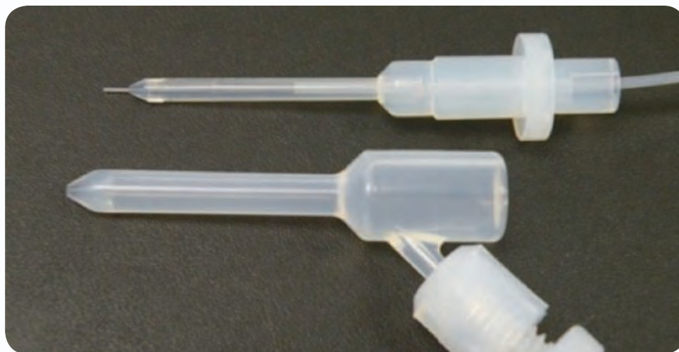
C-Flow nebulizer prior to assembly, showing outer body and inner capillary support.
